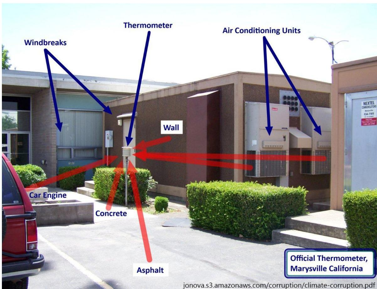
Figure 3: The thermometer at Marysville California<sup>8</sup>. Extra warming from car engines in the parking bays, air conditioner exhaust, asphalt, concrete, a wall, wind breaks, and (see Figure 4) reflections from a steel cell phone tower. [Photo](#) courtesy of Anthony Watts and [www.surfacestations.org](http://www.surfacestations.org).
