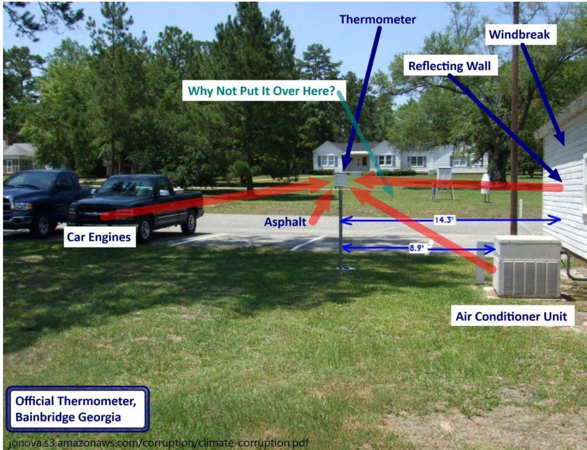
Figure 2: There is a better site on the grass just across the car park, so why is the thermometer near the air conditioner, car engines, asphalt, and reflecting windbreak? [Photo](#) courtesy of Anthony Watts, [www.surfacestations.org](http://www.surfacestations.org) and Joel McDade.
