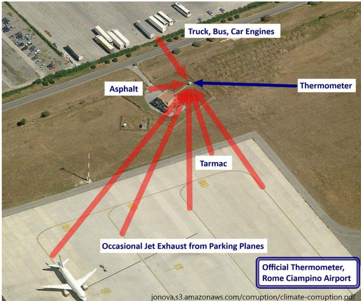
Figure 11: This official thermometer gets some blasts of jet exhaust from parking planes, as well as from several heat sources within 30 meters (100 feet). [Notes](#). [Source](#).
