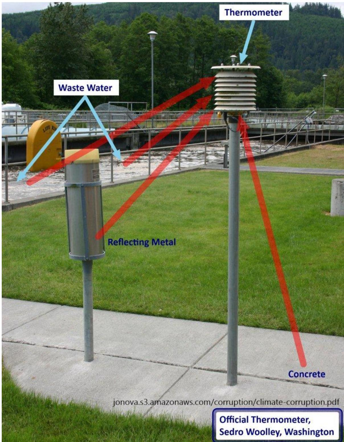
Figure 6: This official thermometer is warmed by the decomposing organic matter in the waste water (the previous figure, of different tanks, shows that waste water is warmer than its surroundings). [Photo](http://www.surfacestations.org) courtesy of Anthony Watts, [www.surfacestations.org](http://www.surfacestations.org) and Don and Liz Healy.
