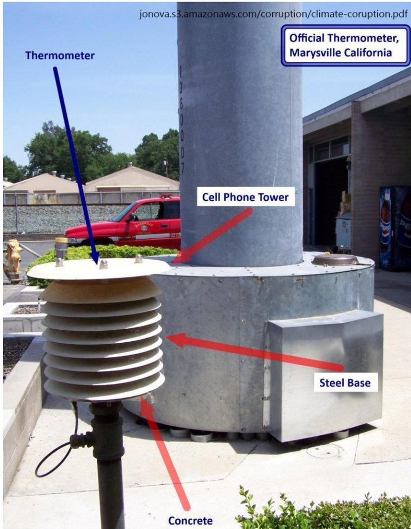
Figure 4: The same thermometer as in Figure 3, viewed from near the air conditioners. Extra warming reflected from a steel cell phone tower. [Photo](#) courtesy of Anthony Watts and [www.surfacestations.org](http://www.surfacestations.org).
